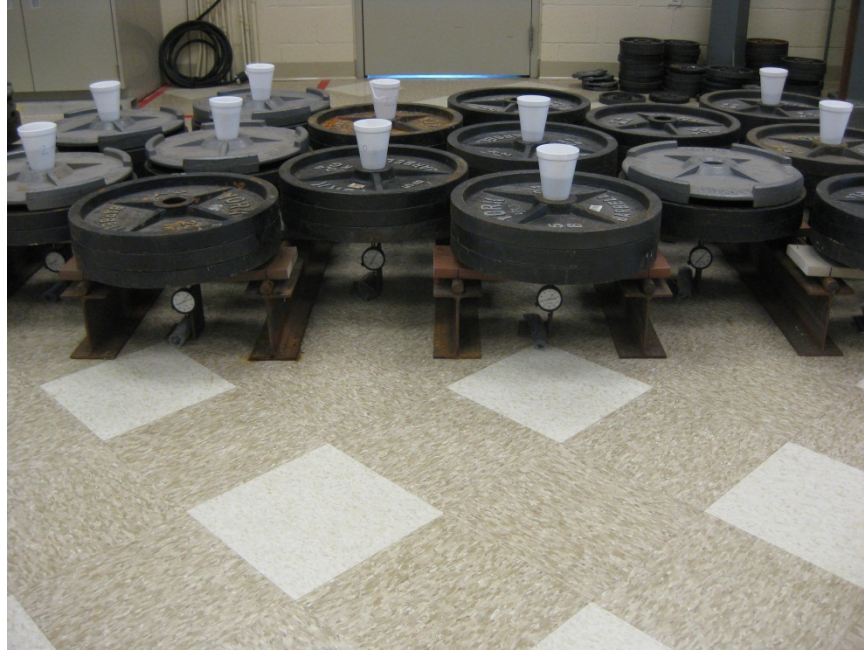
Photo No. 8 Durational Load Test Setup
