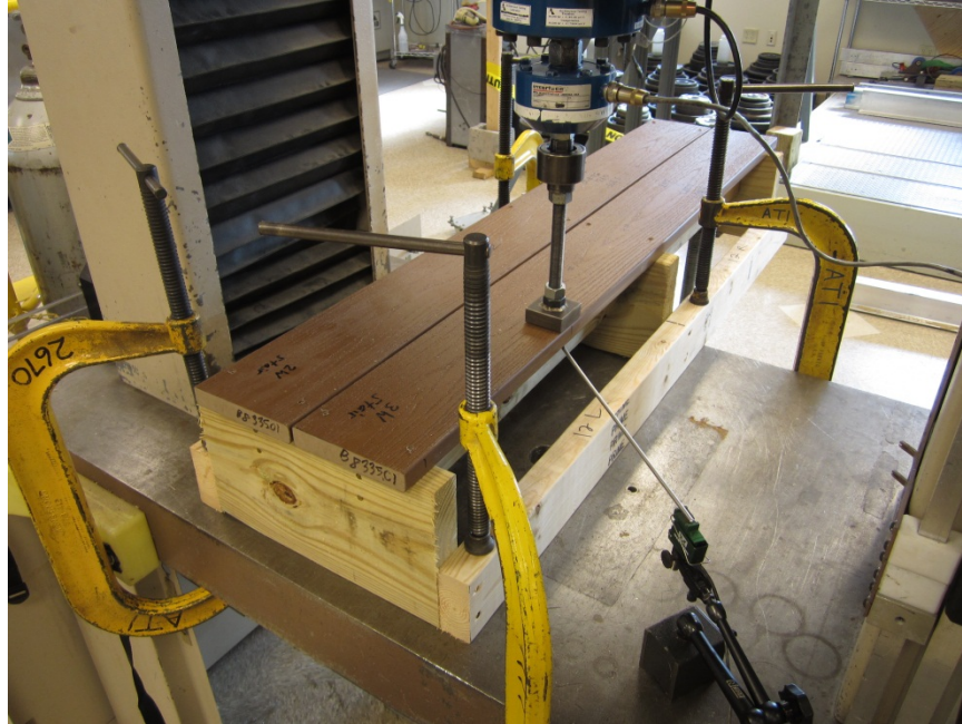
Photo No. 6 Stair Tread Testing at a 24.0 in 2-Span Condition – ASTM D 7032
