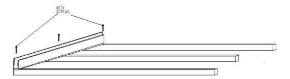
5. Snap the first Gorilla Deck @ Board into the starter strip, pre-drill holes in decking and secure deck board with the # 8 x 1-1/2" stainless steel screws.
