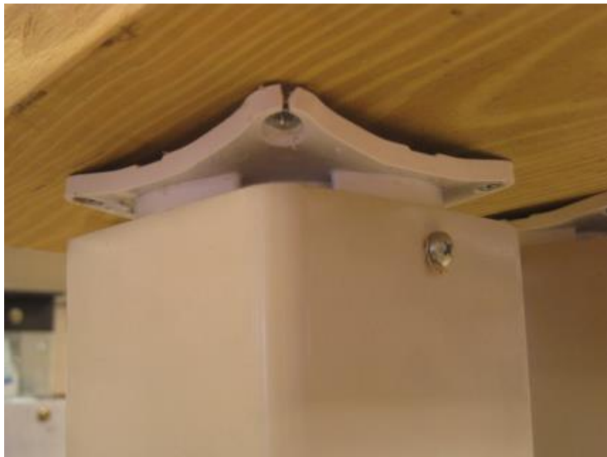
Photo No. 3 Typical Uplift Load Test Failure
