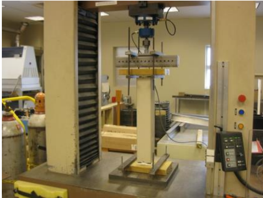
Photo No. 2 Typical Uplift Test Setup
