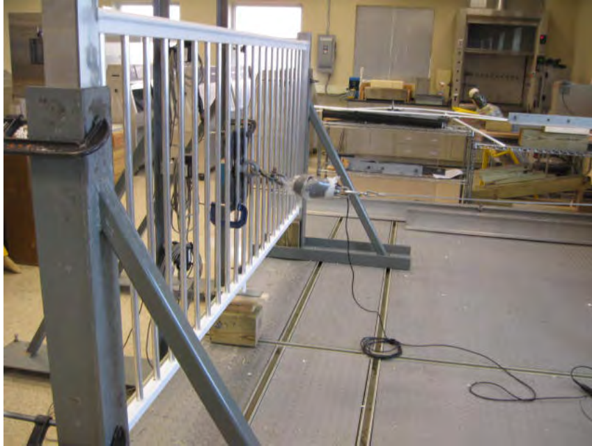
Photo No. 1 In-Fill Load Test at Center of Two Balusters
