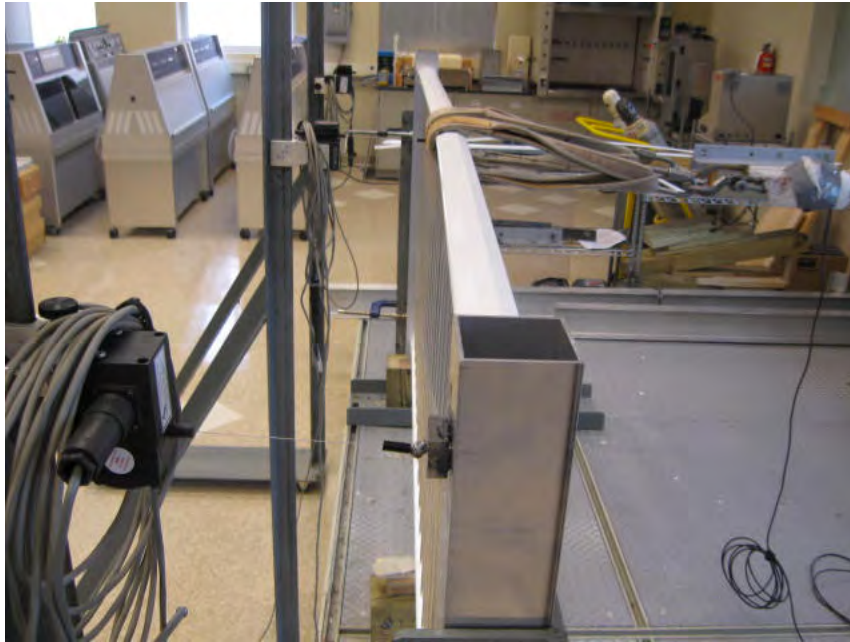
Photo No. 4 Concentrated Load Test at Midspan of Top Rail
