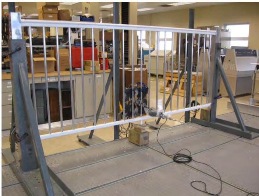
Photo No. 2 In-Fill Load Test at Bottom of Two Balusters
