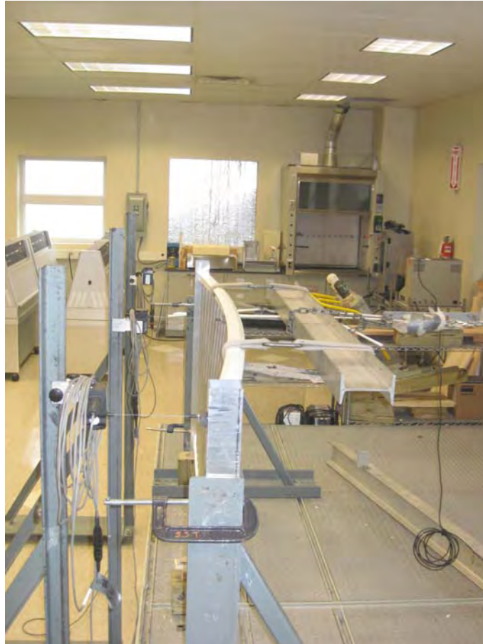
Photo No. 3 Horizontal Uniform Load on Top Rail
